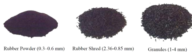
Fig. 1 Difference sizes of crumb rubber used
