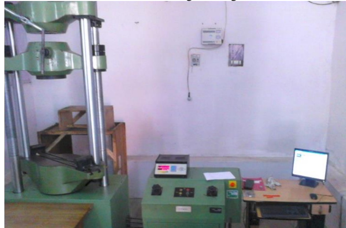
Fig. 3.5 UTM setup for Elongation Test
