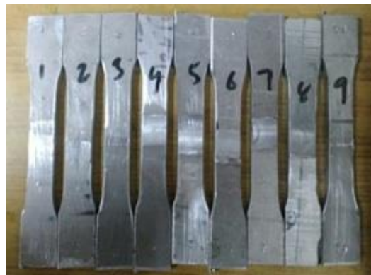
Fig. 3.7 Tensile test specimen before failure
