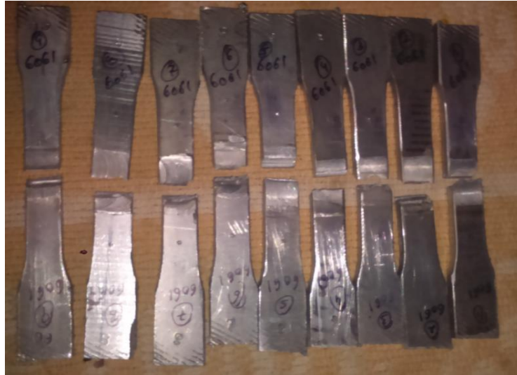
Fig. 3.8 Tensile test specimen after failure
